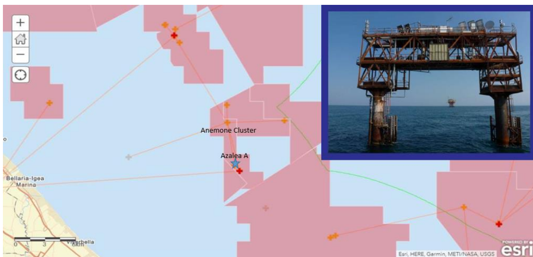
Figure 5. GIS representation of the AZALEA A platform (blue star) and the connection by sealines (orange line) to the nearby platform Anemone Cluster (orange cross). Others orange cross: active platforms; red cross: active platforms connected to land by sealine; pink polygon: exploitation hydrocarbon licenses; green line: 12- nautical mile limit
