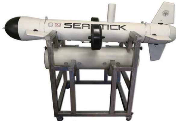
Figure 24. Autonomous Underwater Vehicle equipped with a miniaturized laboratory, developed by Polytechnic of Turin, for autonomous heavy metal detection in seawater near offshore hydrocarbon platforms
