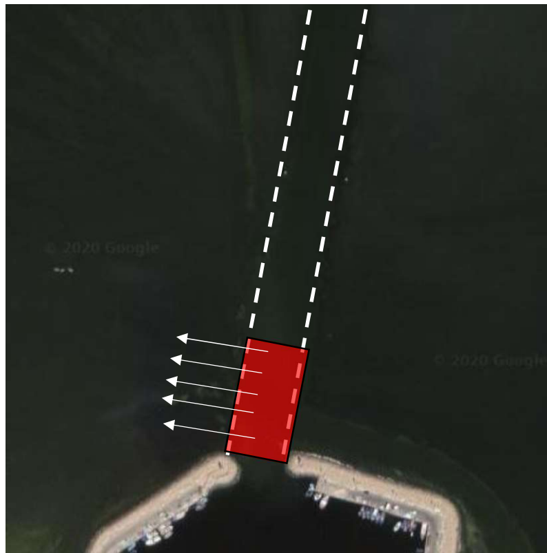
Figure 8. Application of a 5 ejectors plant at the port entrance of Houmt Souk.
